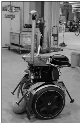
Figure 1. The Segway RMP robot with its primary means of perception, a monocular color camera on a custom pan-tilt unit.
