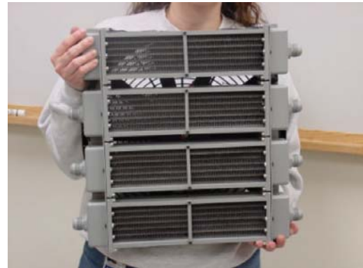
Figure 3: Automotive radiators which demonstrated 33 to 250% performance improvement.
