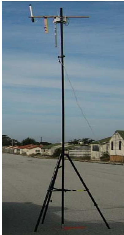
Figure 22. Ground Node Deployment with Tri-Pod
