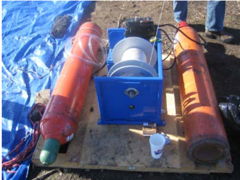
Figure 25. Platform with Helium and Winch
