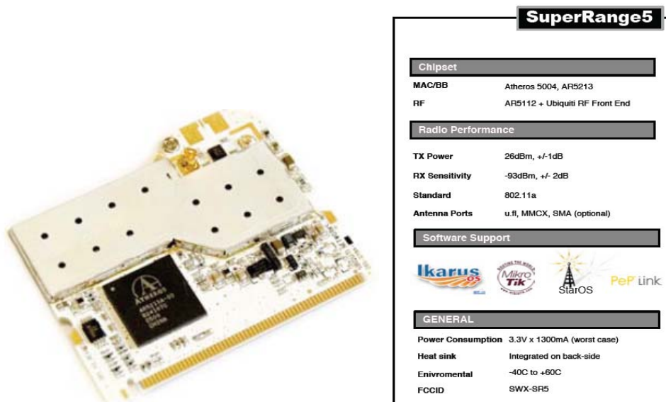
Figure 10. Ubiquiti SuperRange5 Radio (left) and SuperRange5 Specifications (right) (From: http://www.comnet.com.au/Ubiquiti/SR5.htm accessed June 8, 2006)
