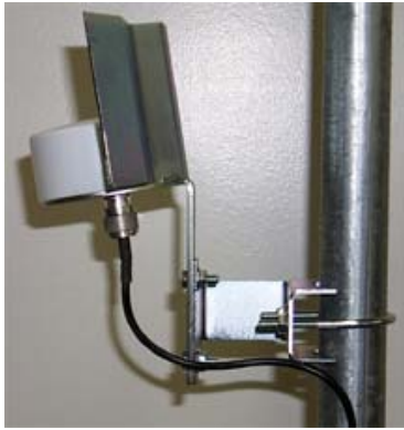
Figure 16. WIFI-PLUS 13dbi Multi-Polar Antenna (From: http://www.wifi-plus.com/images/SpecsSingleSector2.pdf accessed June 8, 2006)
