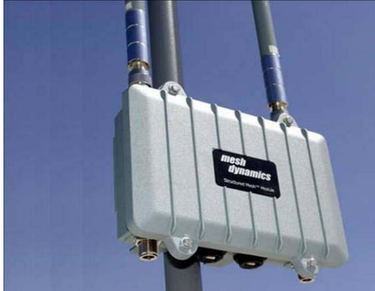
Figure 8. 802.11a/b/g network Mesh Dynamics Unit
