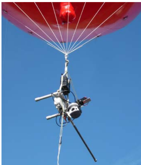
Figure 31. Aerial Node Deployed at Pt. Sur
