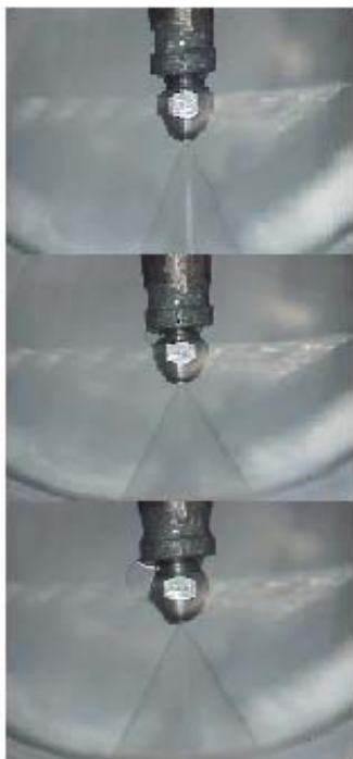
Figure 29. Hago 6 gph nozzle (100°F). From top: 60 psig, 80 psig, 100 psig.
