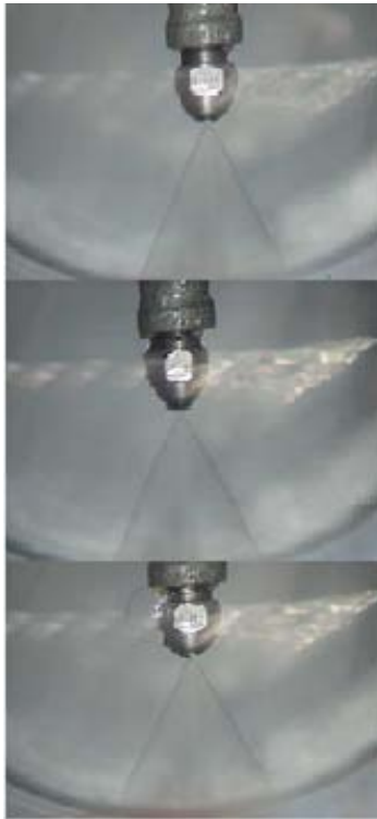
Figure 30. Hago 6 gph nozzle (120°F). From top: 60 psig, 80 psig, 100 psig.
