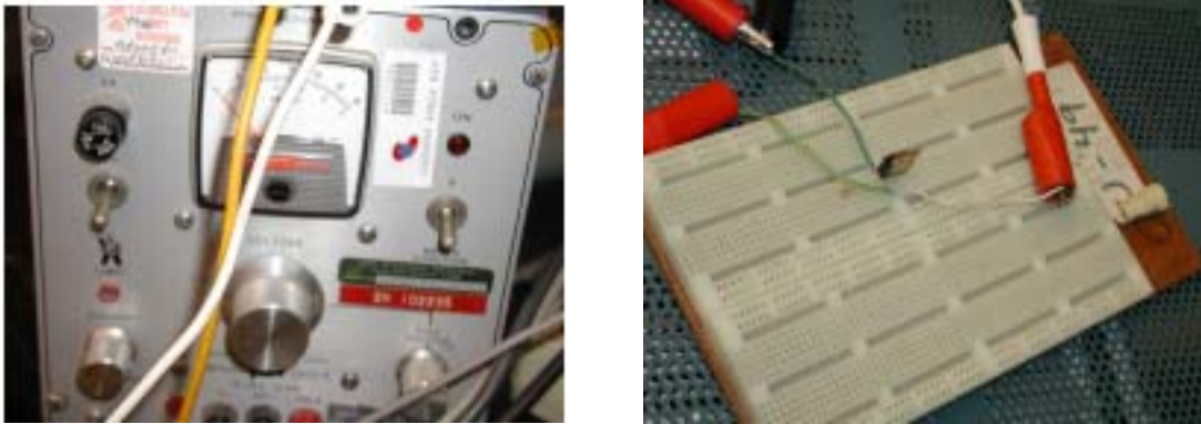
Figure 13 Voltage Source and High Power IGBT.
