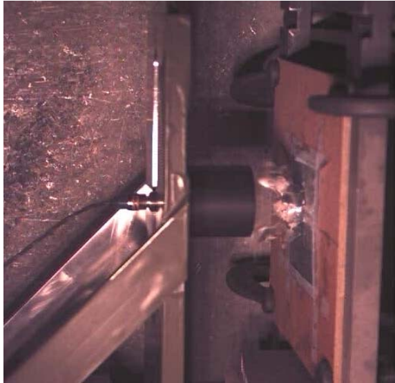
Figure 29. Failure of test 2647. (Again, the rupture of the metal sheet indicated that the strain limit of the material was exceeded significantly.)
