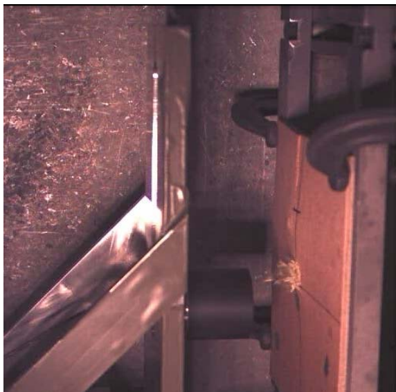
Figure 30. The impact point is well above the position of the 0.75-inch metal disk in test 2648. (The impact does not dislodge the tape, indicating that a smaller area might have a chance of surviving the high differential strain environment of the ballistic test.)
