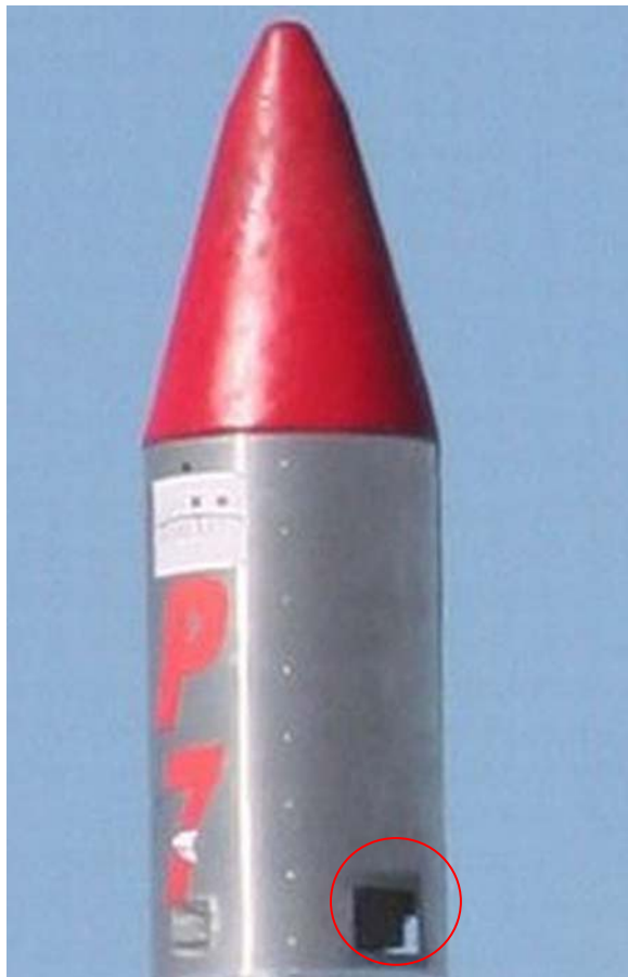
Figure 5. Close-up View of P-POD Deployment Port at the Aft End of the P-7 Interstage
