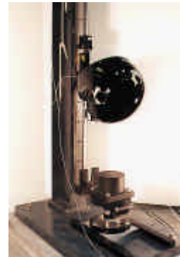
Motorcycle helmet test device
