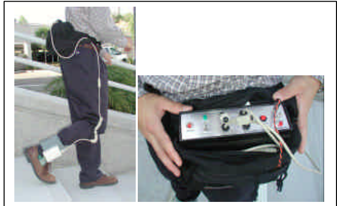
The portable F-scan System is comprised of foot sensors and a data storage pack.
