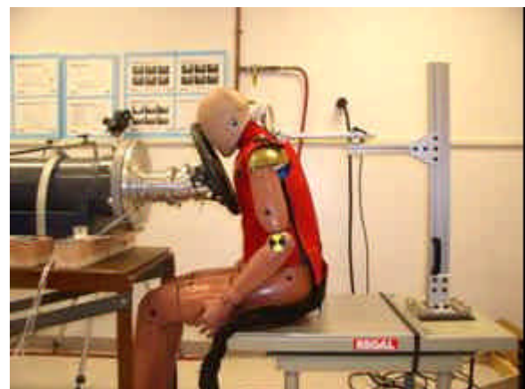
THOR dummy seating in front of ATS
