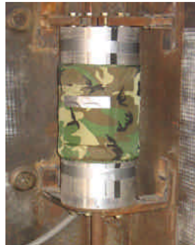
FBTD with surrogate armor in field test
