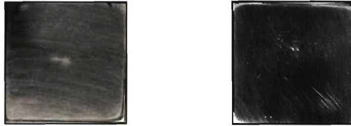
Figure 20. Photographs of test coupons following 12 hours exposure to cavitation: alloy 686 at a separation distance of 0.03 inches with no Arizona Test Dust (left), and alloy 686 at a separation distance of 0.03 inches with Arizona Test Dust (right).
