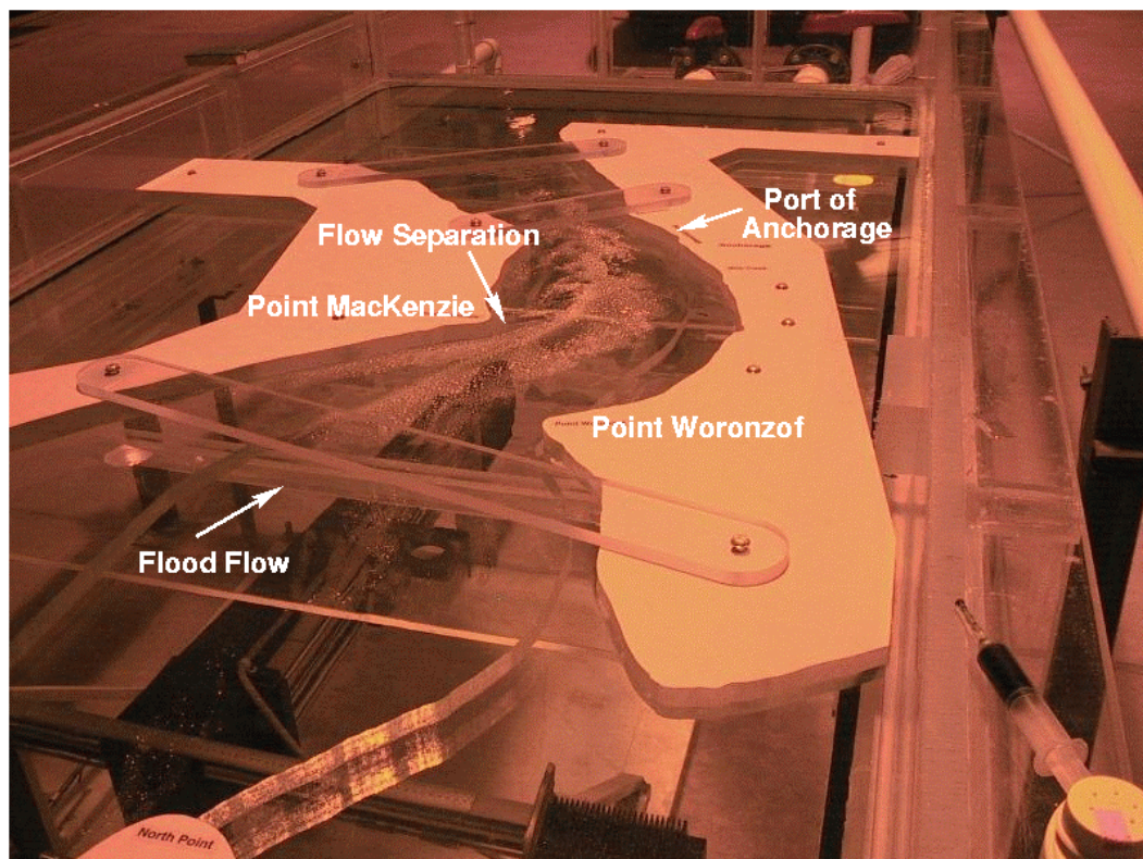
Figure 4. Idealized model of a portion of Cook Inlet, AK, during flood flow
