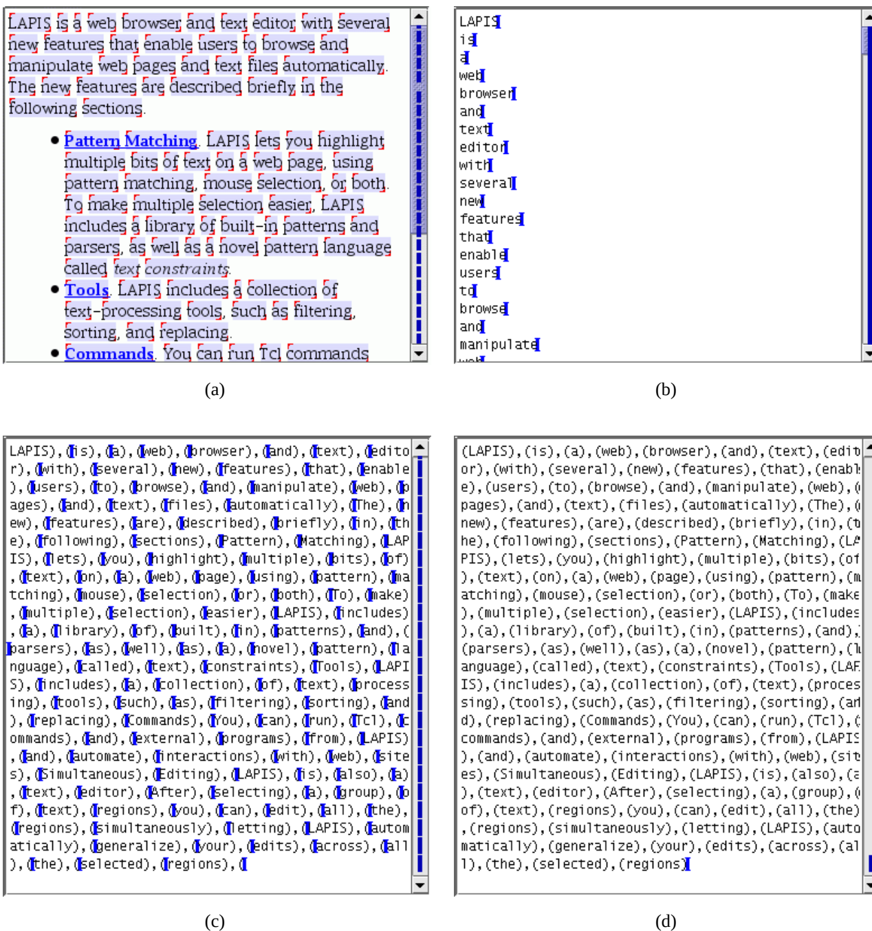
Figure 8.3: Using copy and paste to extract a selection. (a) The selection (WORD) is copied to the clipboard. (b) After making a new document with File/New, the clipboard is pasted, leaving an insertion point after each pasted region. (c) The user deletes the linebreaks that were inserted by default, and types ), ( instead. (d) The user fixes up the boundary cases, before the first and after the last extracted region.
