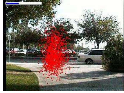
Fig. 9. Particle filter tracking: The position of particles are represented by small dots, and the horizontal bar on the top-left corner shows the number of particles being used.
