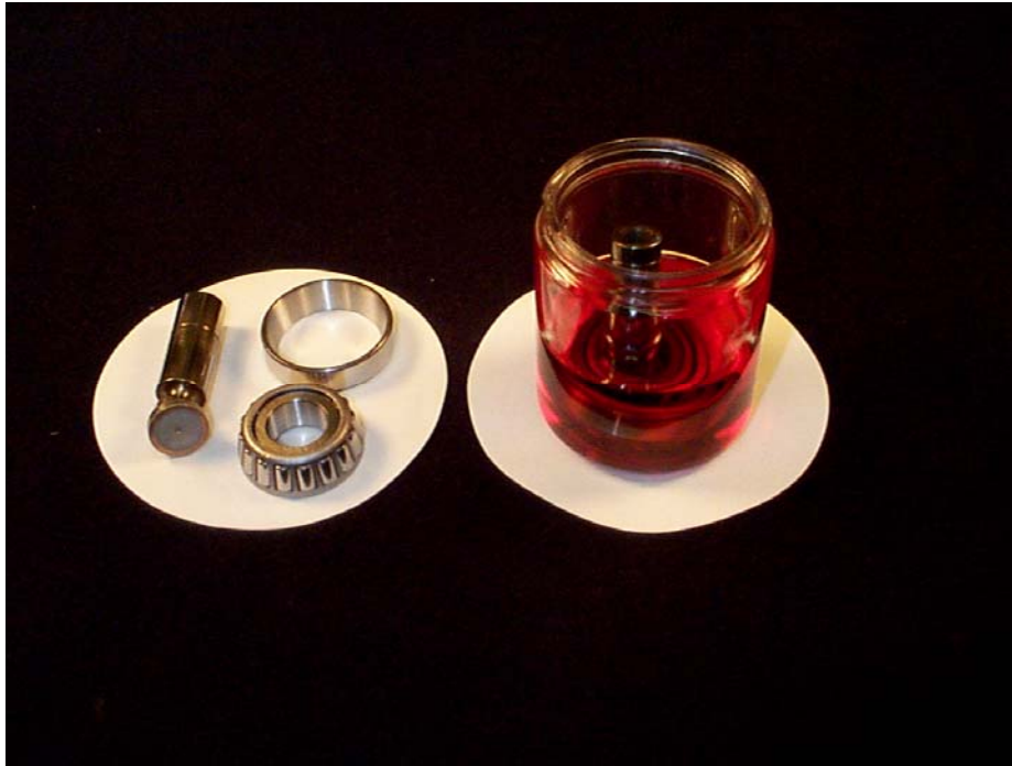
Bearings and pistons shown in and out of a fluid filled storage jar.
