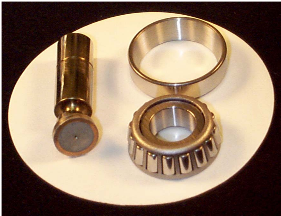
A close up view of the bearing and pump piston
