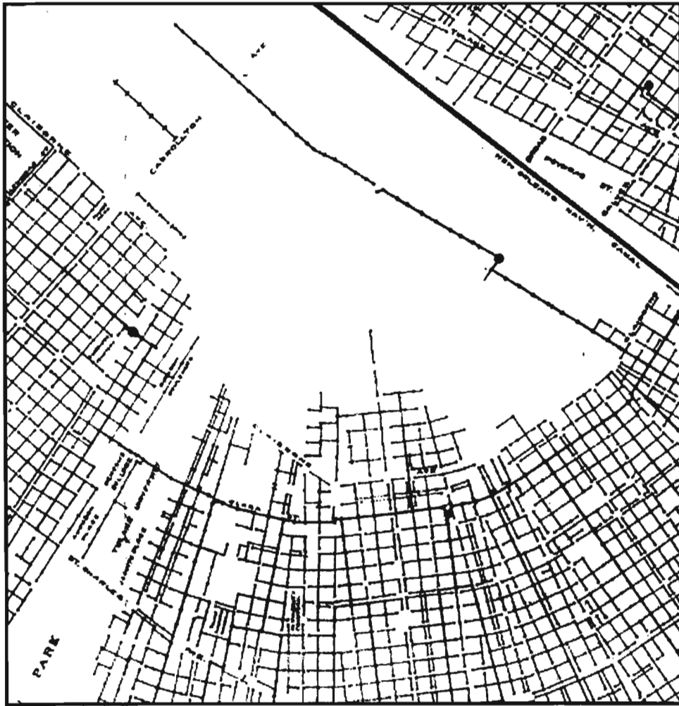
Figure 13. Sewerage connections in the project area ca. 1915. Only those streets closest to Napoleon and Claiborne had city sewage (Sewerage and Water Board, Semi-Annual Report 1915).
