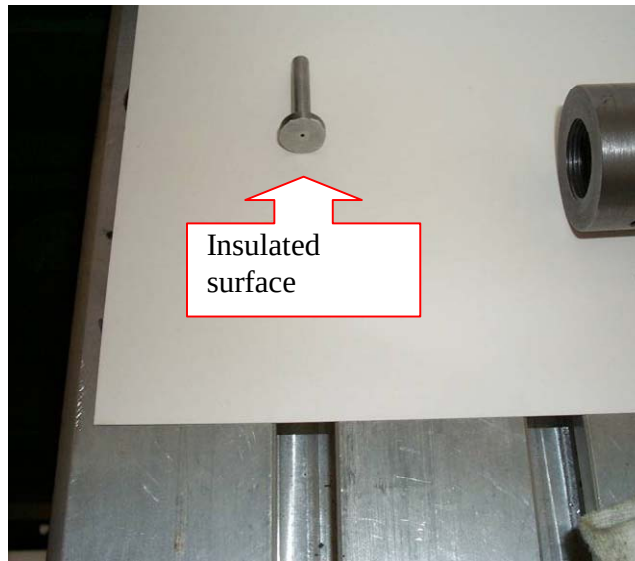
Figure 7. Tape-insulated surface of pin body.
