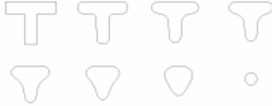
Figure 3.3: Generator of symmetric random walk on the tangent direction implemented on the level set function u(x, y) for a T shape. The tangent direction is estimated directly from the level set function : \theta_T = \tan^{-1} \left( \frac{-u_x}{u_y} \right) . The level set function is on a 250 \times 250 grid, \delta t = 0.25 .
