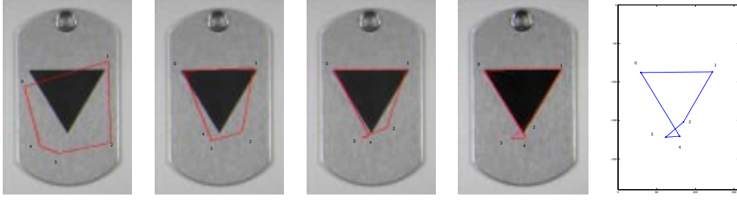
Figure 4.7: We demonstrate that flow (4.6) may become degenerate without an additional constraint on the motion of vertices.
