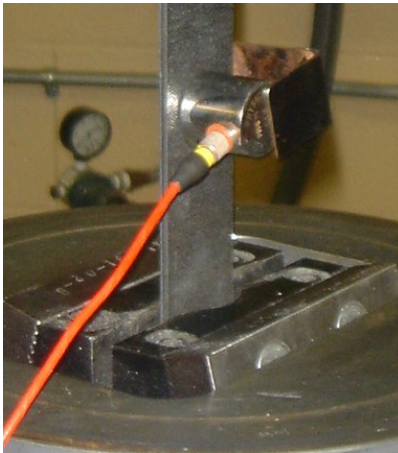
Figure 190. Acoustic sensor attached to specimen.
