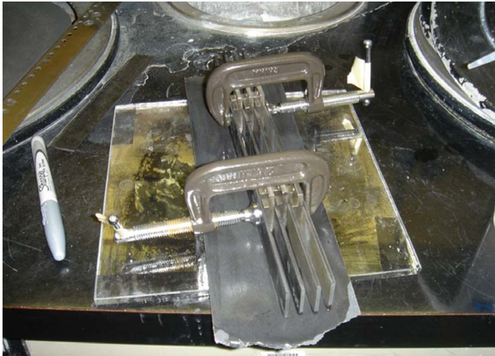
Figure 58. Clamped specimens in configuration used for replication of diffraction grating.
