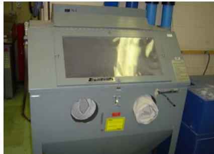
Figure 45. Machined panels were sand blasted for final surface preparation.
