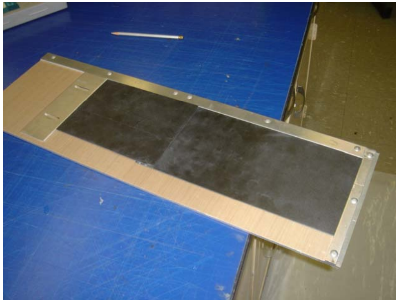
Figure 23. Jig used during adhesive curing.
