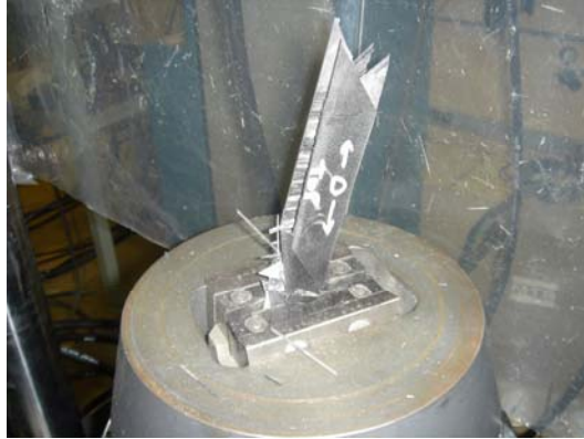
Figure 193. Fractured virgin specimen 1 in MTS machine.
