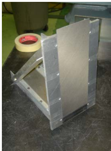
Figure 14. Panel fixed to Apparatus used to create scarf
