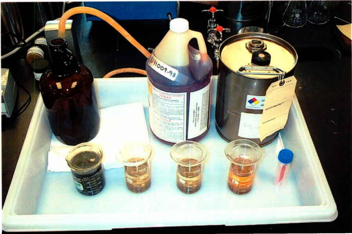
Figure 4. Sample Preparation for Biocide Efficacy Test
