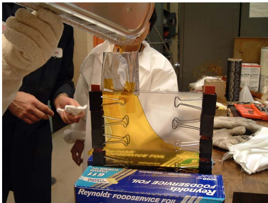
Figure 9. Transfer of the BMI 5250-4 into the Mold
