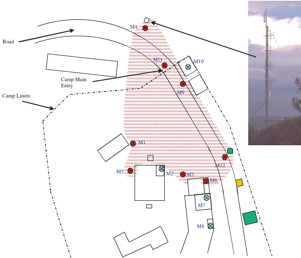
Fig 3. A sketch of the camp and the surrounding area showing the points of measurement (M1- 12) and the area in red where the RF radiation exceeds the Greek reference levels. The photo shows the radio station antenna causing the high radiation levels.
