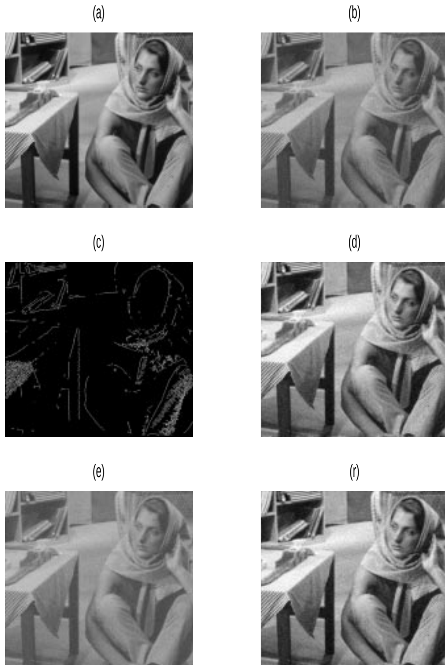
Figure 5.13: (a) Original bar girl ; (b) bar girl plus Gaussian noise; (c) Edge points extracted from noisy image; (d) Filtered result from the Gaussian noise corrupted image; (e) bar girl plus Laplacian noise; (f) Filtered result from the Laplacian noise corrupted image;
