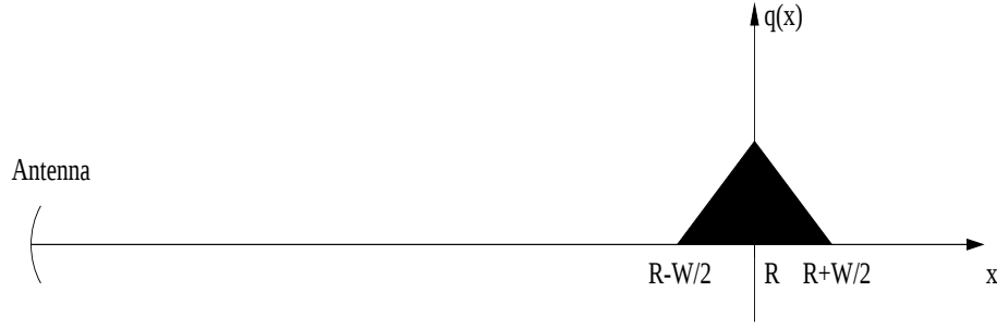
Figure 2.3: Simplified geometry for range processing.
