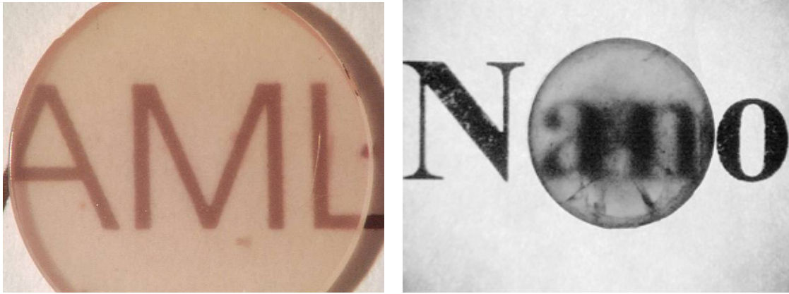
Figure 12: Translucent yttria disks. Left: Made from Nano-1 powder (0.9 mm thick). Right: Made from Nano-2 powder (2.0 mm thick).
