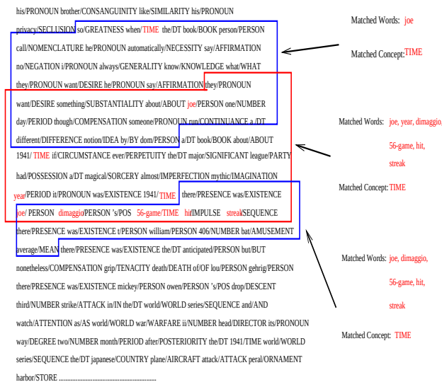
Figure 3: An example of applying dynamic sliding window techniques: Three adjacent optimally formulated windows are shown. The top window segment with four sentences contains the query concept “TIME” and matching word “joe.” The second window with five sentences contains the query concept and six keywords. The last window with two sentences contains the query concept and five keywords.
