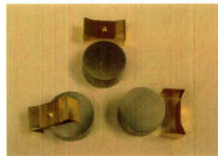
Figure 5: Illustration of galvanic couple assembly.
