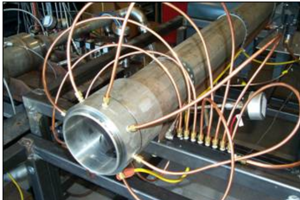
Figure 5. Liquid propane injection.
