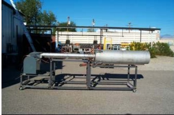
Figure 3. Nonexpendable portion of the controlled heat flux combustor.
