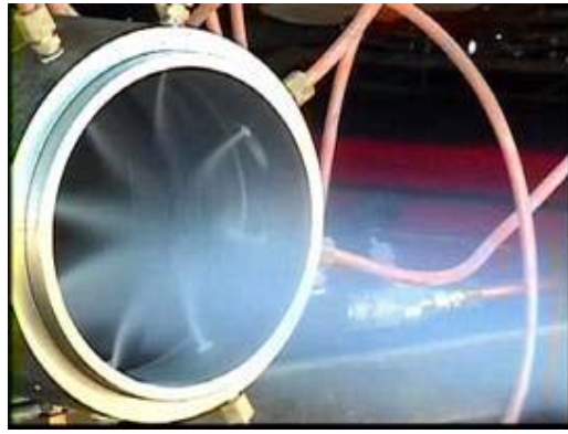
Figure 6. Liquid propane injection.
