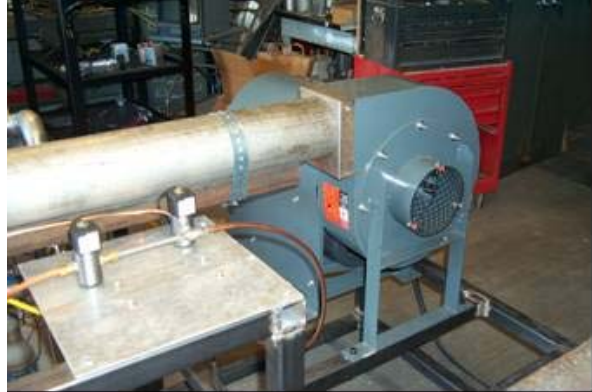
Figure 4. Controlled heat flux combustor blower fan.
