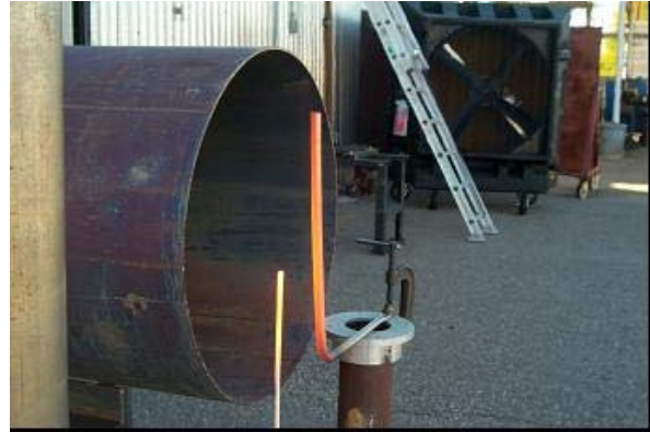
Figure 12. Controlled heat flux combustor operating at 1400°C.
