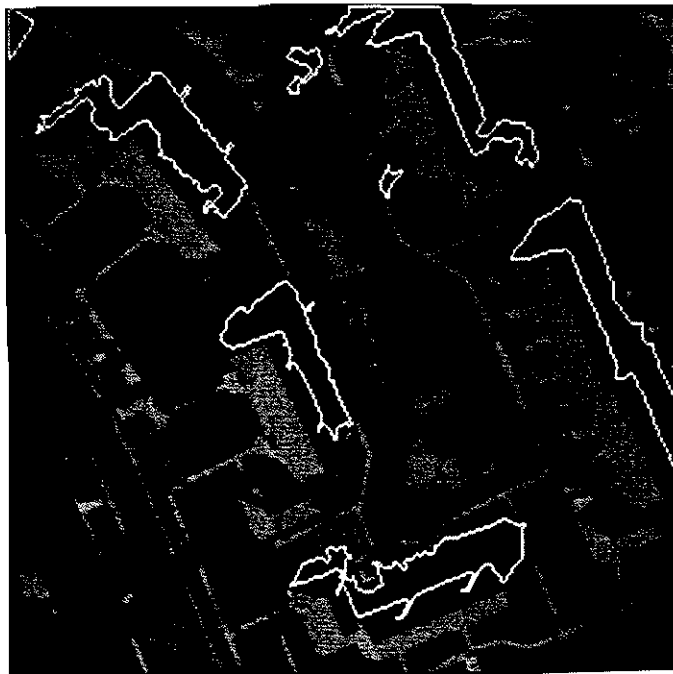
Figure 16: Shadow region boundaries extracted from the large region by applying simple criteria based on alignment with the sun, intensity, and size.
