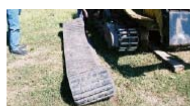
Picture 53 – Track removed
