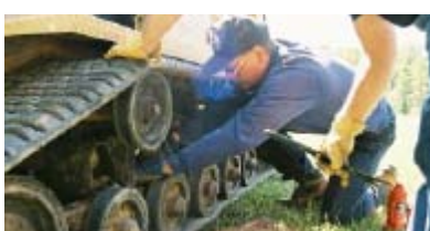
Picture 52 – Releasing rear axle tension
