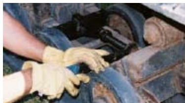
Picture 51 – Adjusting track length
