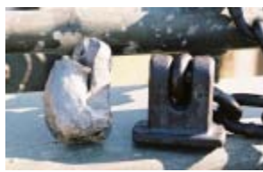
Picture 31 – A worn flail head (left, lost during run) and a new flail head (right)
