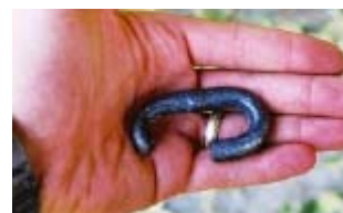
Picture 32 – Broken interlink
