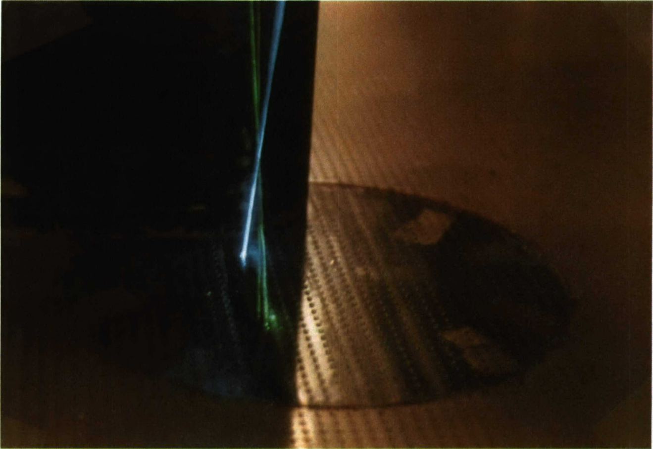
Figure 2.6. Appendage Junction: Laser beams passing through transparent floor through the spacing between the cylindrical roughness elements.
