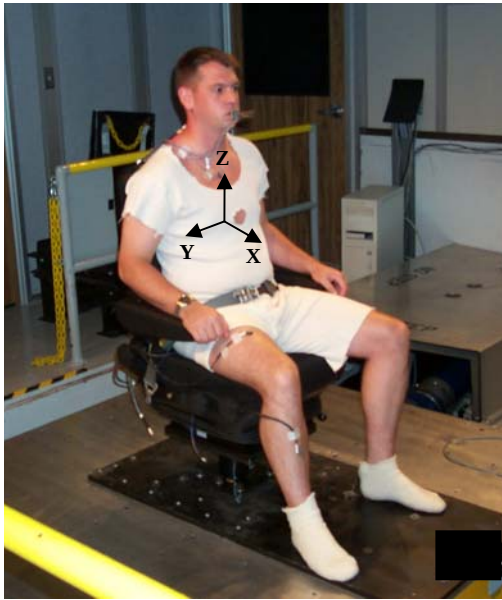
Figure 1. Locomotive Seat Attached to SIXMODE Vibration Table
