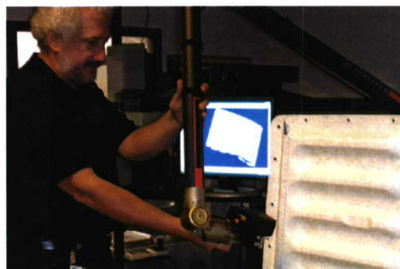
Digital data capture using laser scanner
