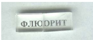
Fig. 2.2.1. The samples of (left) artificial monocrystalline fluorite and (right) Suranskoe cryptocrystalline optical fluorite (SCOF).
