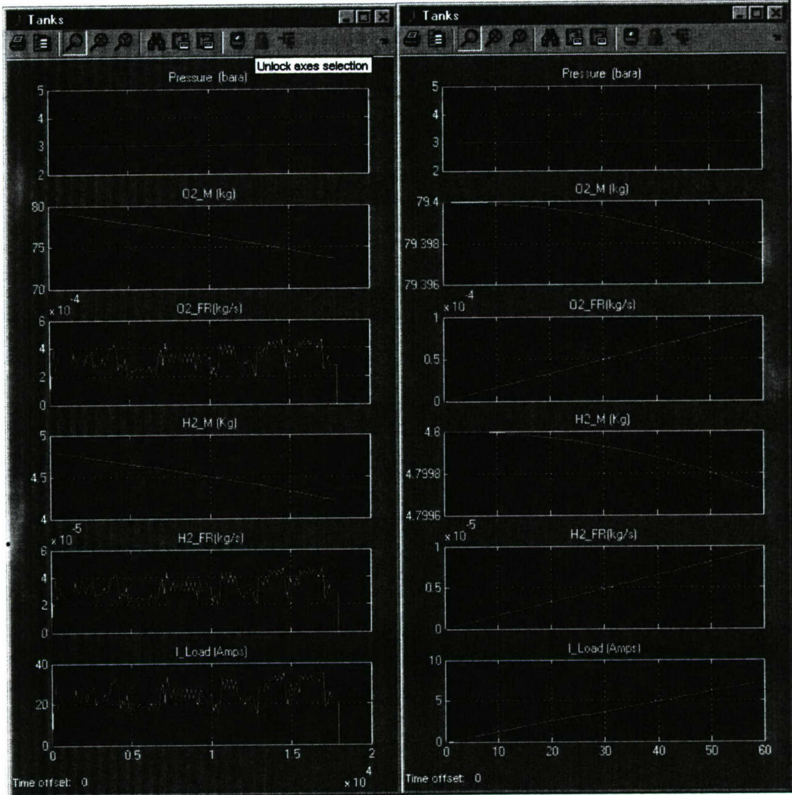
Figure 16: H 2 and O 2 tanks mass and flowrates under a dynamic UUV duty cycle
