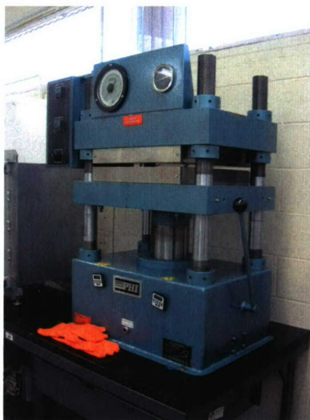
Figure 3.2-10: Manually operated hotpress of 50 ton pressing capacity.
