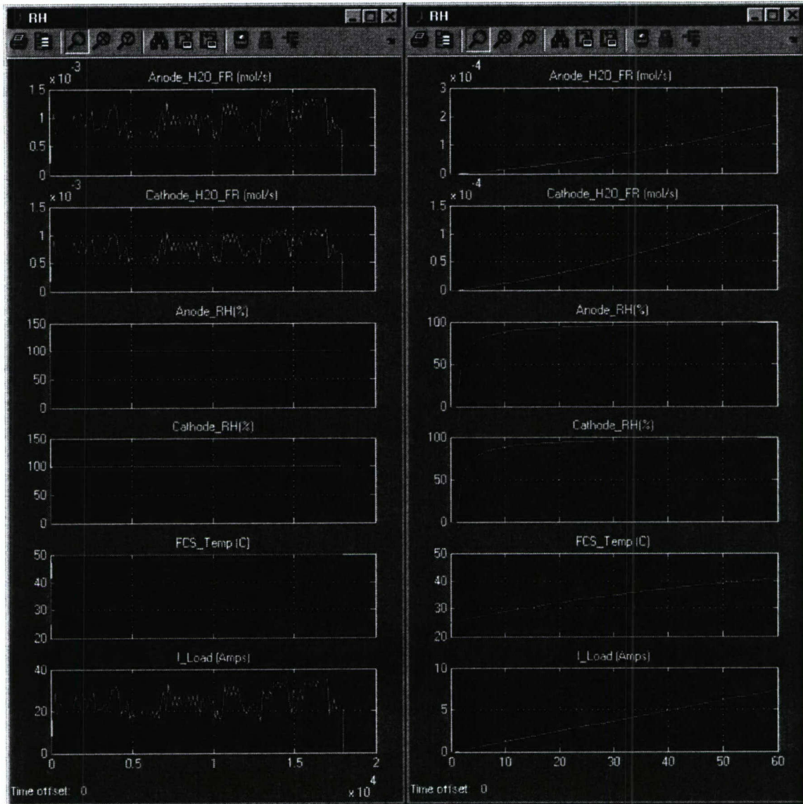
Figure 15: Anode and Cathode relative humidities under a dynamic UUV duty cycle
