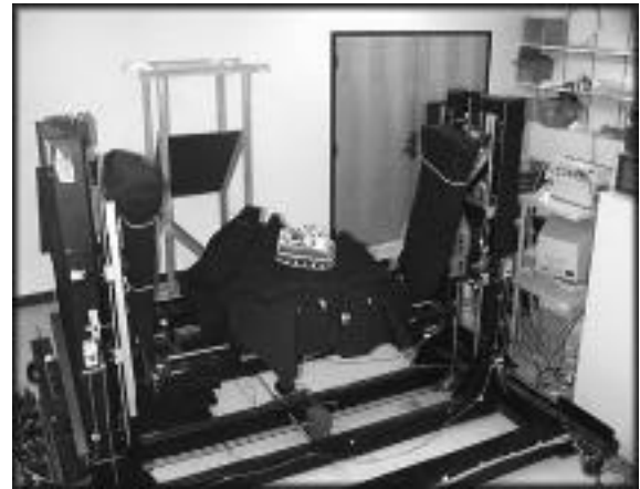
Figure 3. 3DI System 5-Axis Translation Stage (with Target and Calibration Objects).
