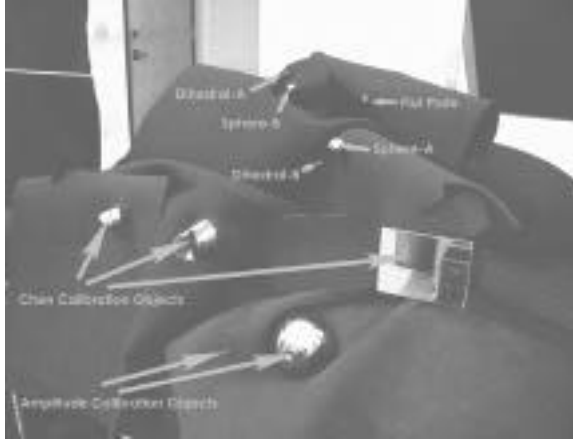
Figure 4. Calibration Objects Mounted on Target Stage.
