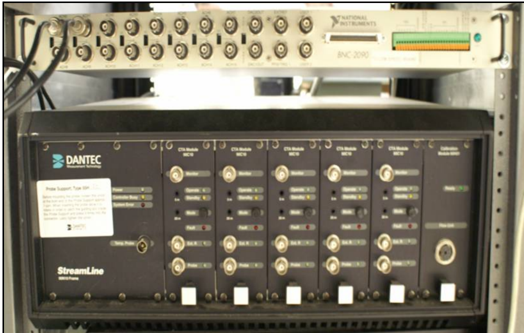
Figure 2- 11 90C10 CTA Modules with BNC 2090 ADC board
