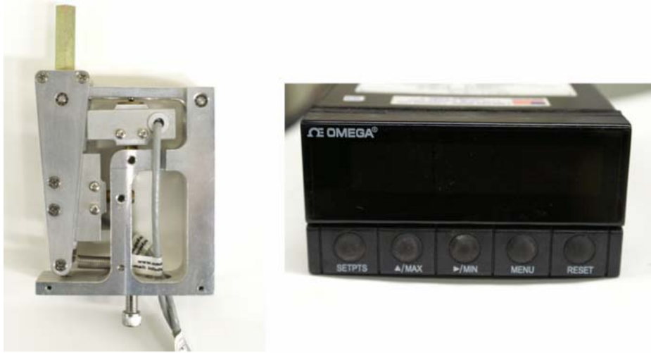
Figure 3- 8 OMEGA LC703-10 load cells with a DP41-S-A conditioner
