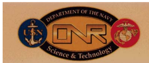
Figure 7. Photograph of the ONR symbol (actual size 1.5 in. \times 0.75 in.) taken through a thick film ( \sim 50 \mu\text{m} ) of polymer 7 supported on a glass slide. The film was doctor-bladed from a 20 wt % solution of cyclohexanone.
