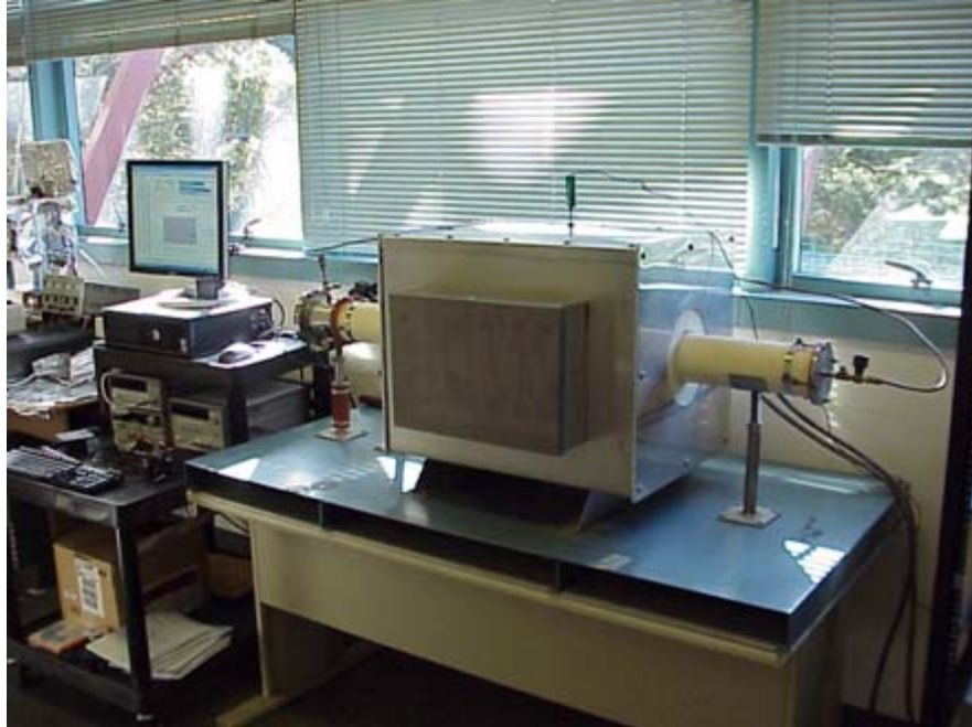
Figure 3. Picture of tube furnace and associated data logging computer.
