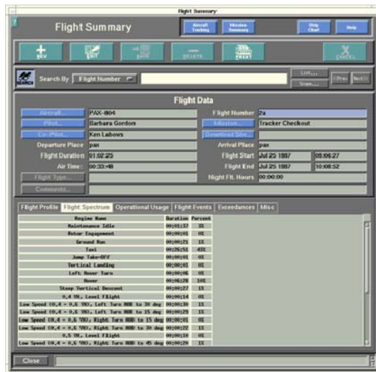
Figure 2. An Example of the Ground Station Screen of a Flight Summary and Flight Spectrum Report for a Single Flight (From Goodrich, 2001)
