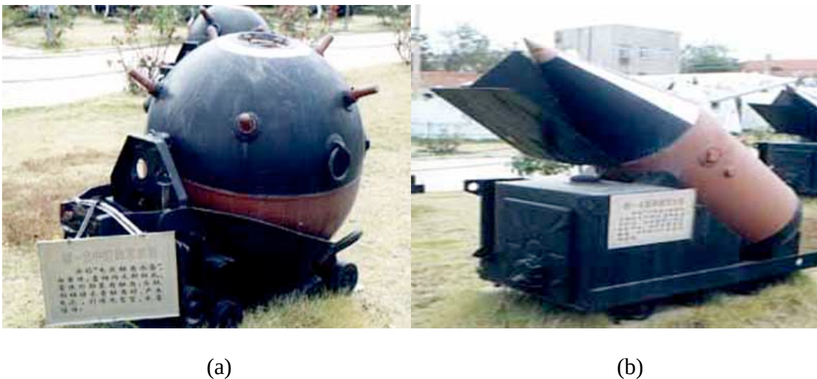
Figure 2. (a) M-2 moored mines carried by surface ships designed to block seaport and routes to attack ships. (b) M-4 acoustic moored mine has strong resistance to the background noise and is designed to attack medium sized surface ships and submarines. (From SinoDefence.com)
