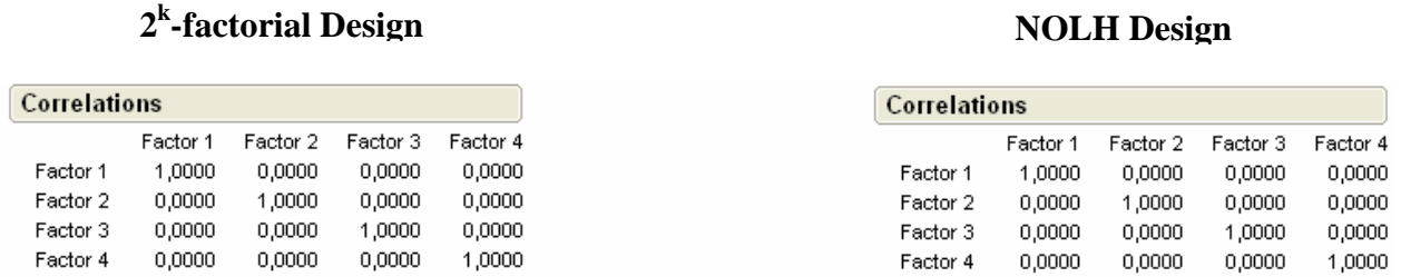
Figure 15. Comparison of the correlation matrices of a 2^k -factorial design and NOLH design.
