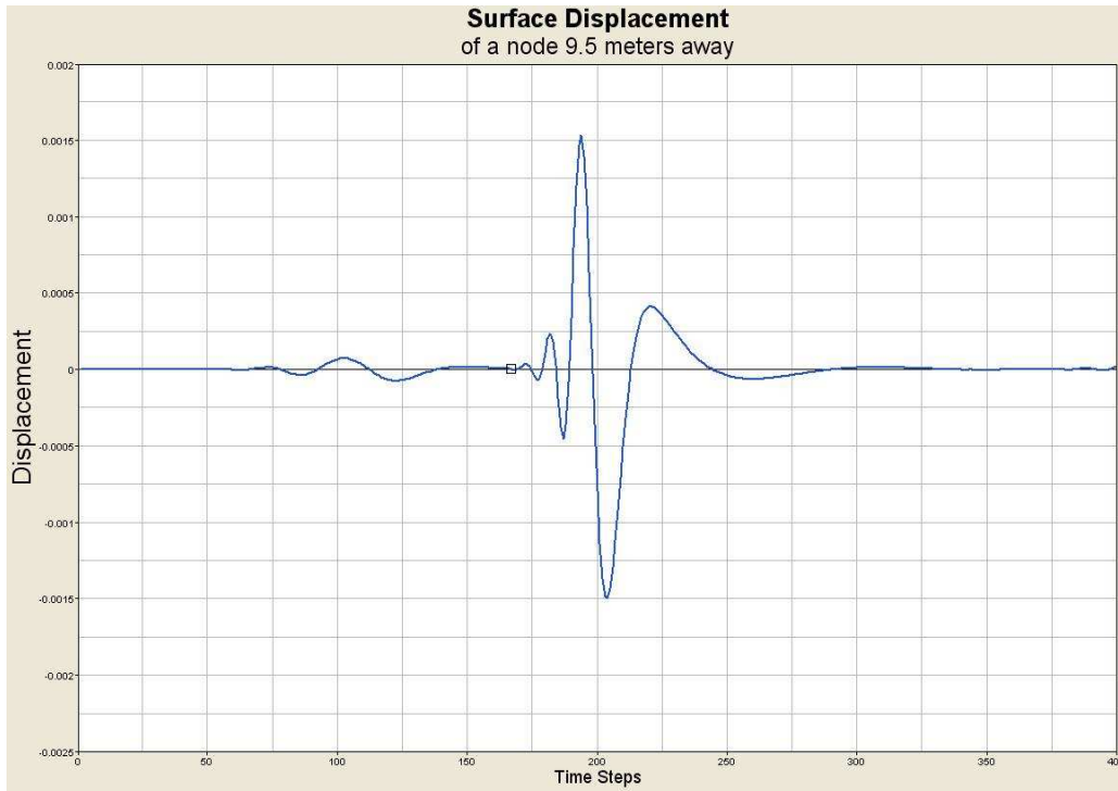
Figure 37. SAFE-T vertical displacement results with PML present. Notice the smooth transition to rest on the surface after the wave passes. Time is represented in \Delta t time-steps which are 0.0005 seconds apart. The medium is the same as in figure 36 which exhibits a compressional wave speed of 1600 meters per second, a shear wave speed of 100 meters per second, and a Rayleigh wave speed of 95 meters per second.
