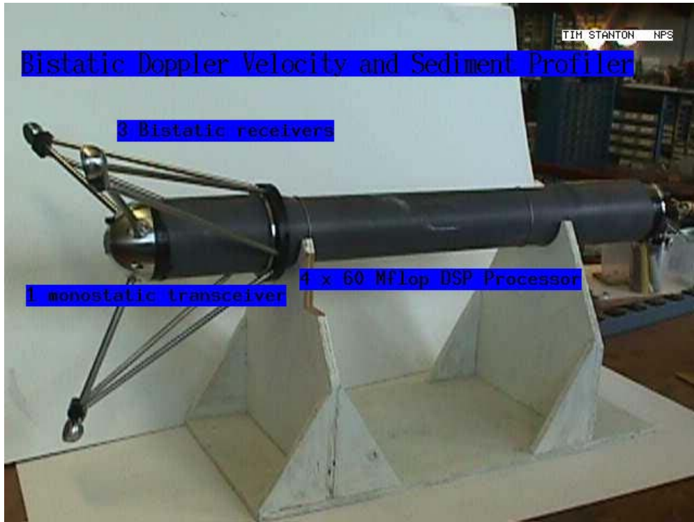
Figure 6. Bistatic Coherent Doppler Velocimeter (BCDV) developed at NPS by Dr. T.P. Stanton and the Ocean Turbulence Research Group. The BCDV directly measures instantaneous sediment concentration and velocity through 1 m of water with 1 cm resolution.
