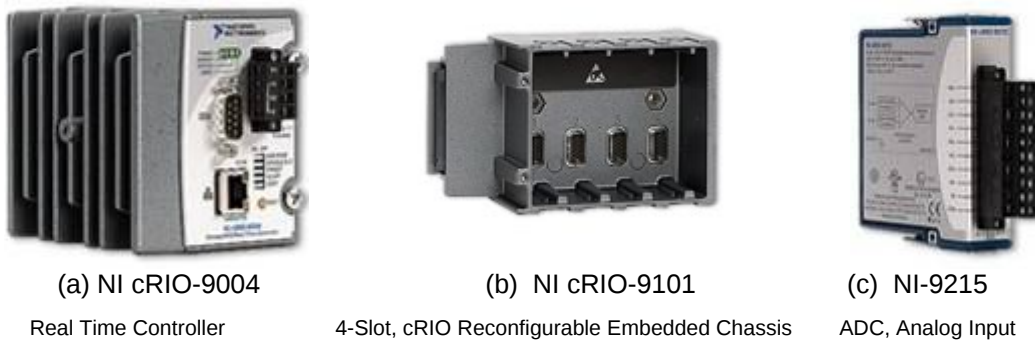
Figure 26. NI Modular Systems Used for Demonstration Array (From [17-19]).
