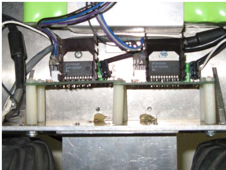
Figure 13. Both motor controllers mounted on the underside of AGV.
