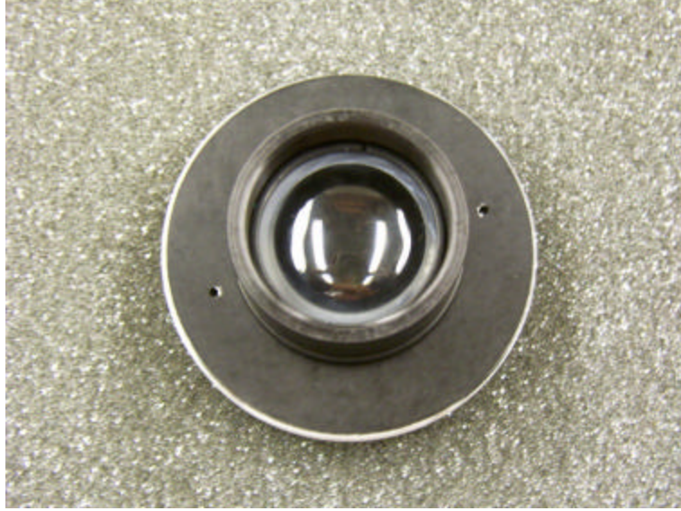
Figure 23. Picarin lens used for the microbolometer camera.
