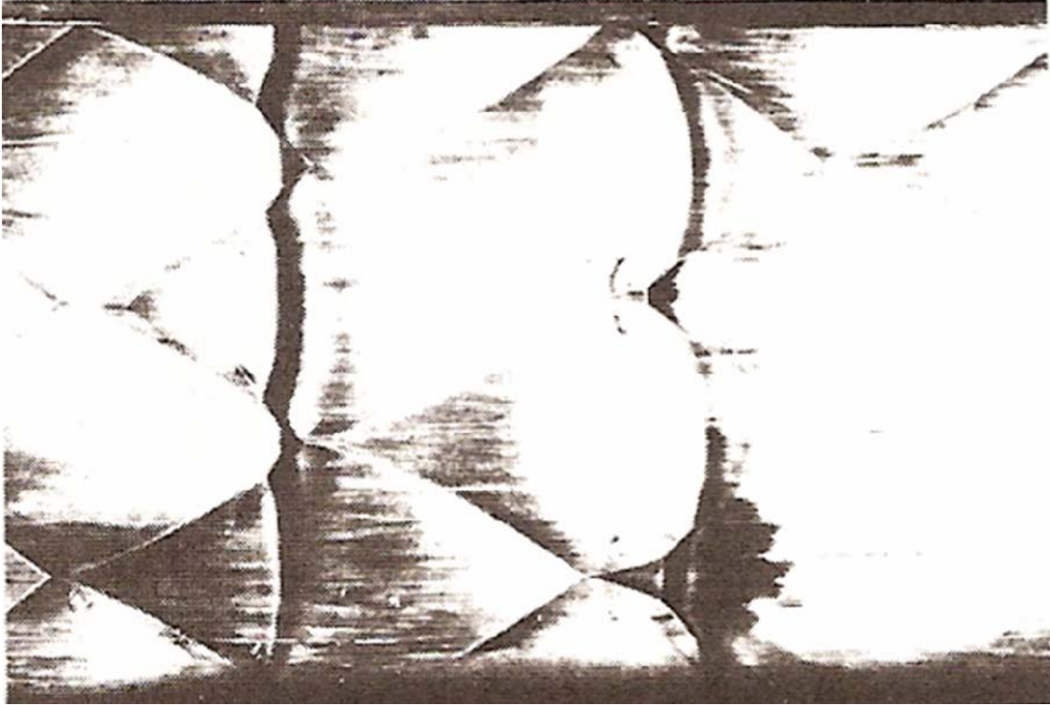
Figure 6. Image of Three-Dimensional Nature of Detonation Wave (From [3]).
