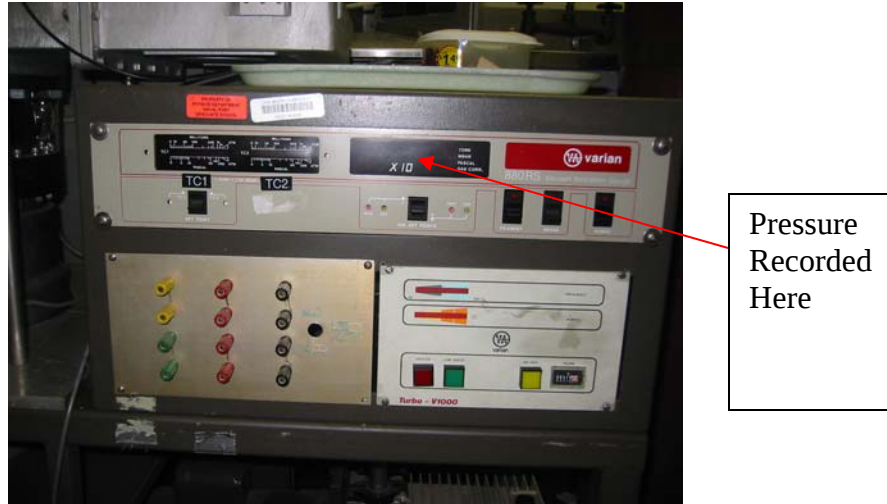
Figure 21. Varian 880RS Vacuum Ionization Gauge
