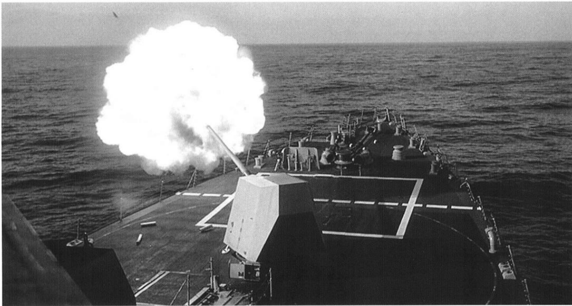
Figure 8. The MK 45 Mod 4 test firing a conventional round (From Annati, 2003).
