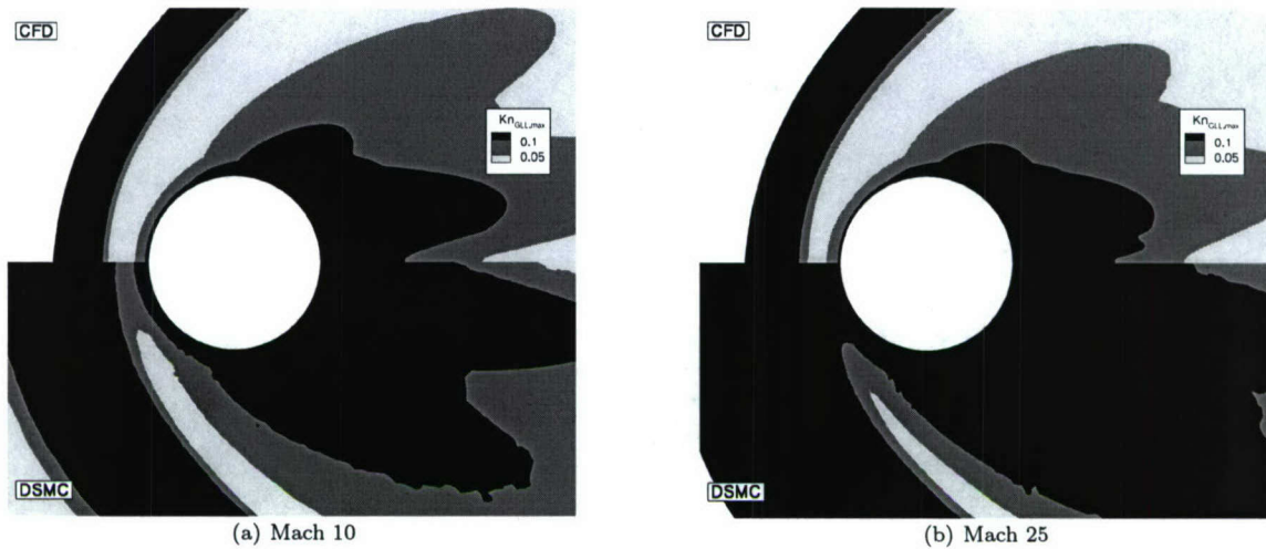
Figure 14. Kn_\infty = 0.05 Kn_{GLL} for Mach 10 and Mach 25. Light gray regions correspond to Kn_{GLL} < 0.05 , dark gray regions correspond to Kn_{GLL} < 0.10 and black regions correspond to Kn_{GLL} > 0.10 . Continuum breakdown is predicted in much larger regions than previous cases. The DSMC method predicts larger regions where continuum breakdown exceeds the critical value of 0.05, with an even larger region predicted for the Mach 25 case. cylinder.
