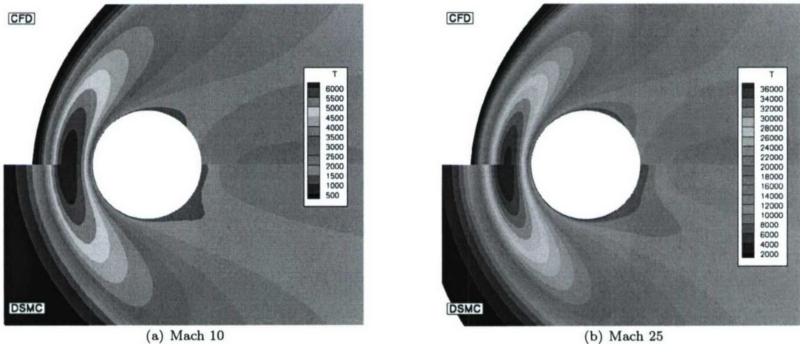
Figure 15. Kn_\infty = 0.05 temperature field for Mach 10 and Mach 25.
