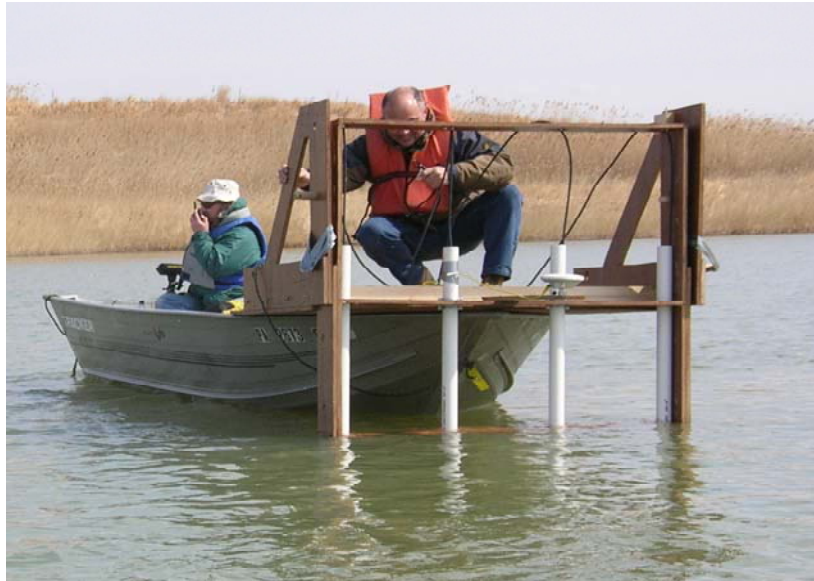
Figure 4. CTC shallow water UXO detection platform - deep deployment.
